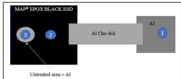
Two coupons were used for each thickness samples of MAP® EPOX BLACK ESD: 7 µm and 14 µm. The measurements were carried out between #1 and #2 areas (“Measure 1–2” in Table 5) and between #1 and #3 areas (“Measure 1-3” in Table 5). For each coupon, three measurements were done. The average measurements are listed in the table below.
