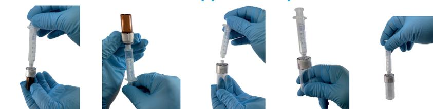
Attach the syringe by screwing it onto the hardener tip. Take up all of the hardener by sucking up with the syringe. Screw the syringe onto the base and inject the hardener. Mix by sucking up the contents of the mixture. Unscrew the Viale syringe from the base.
