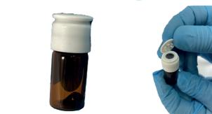
Remove the cover from the vial Ø10 mm of the hardener
