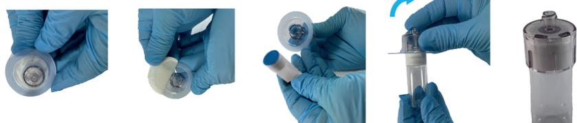
Remove the cover of the Ø20 mm striker and fix it on the Ø10 mm vial of the hardener. Remove thestricker pin protection.
